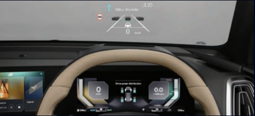
31.24cm (12.3") HD Display Instrument Cluster with Head-up Display Unit
