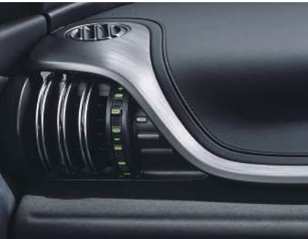
Dumbbell-style Air Conditioning Vents
